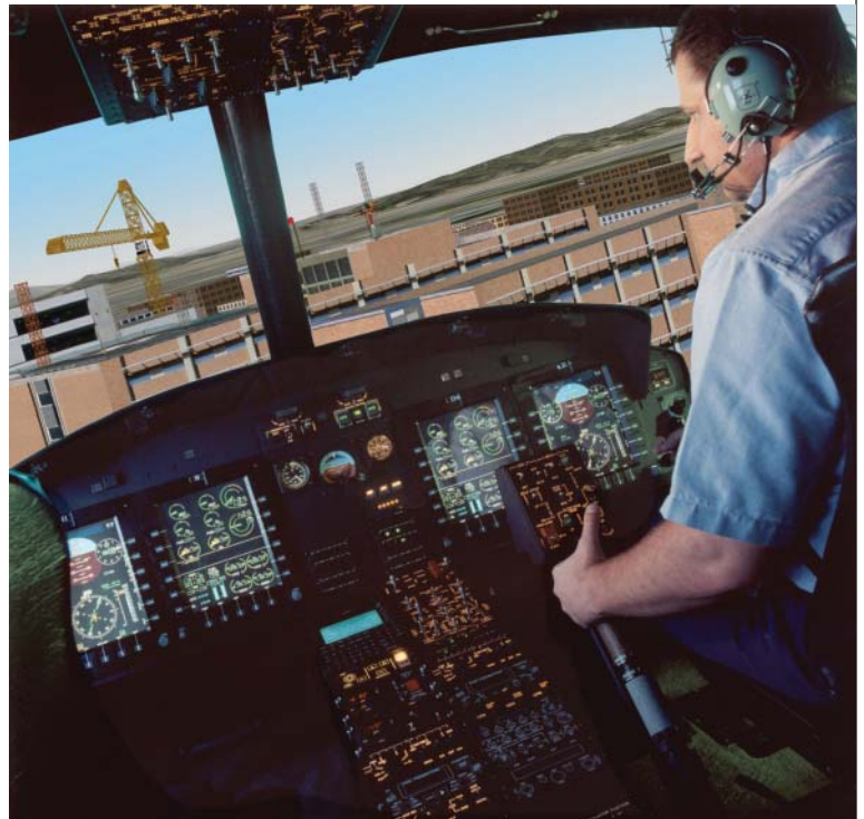
Above: Bell 412 FTD with TruVision and custom database
