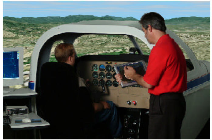
Frasca TruFlite™ with wide cockpit and 170 degree TruVision™ visual system
