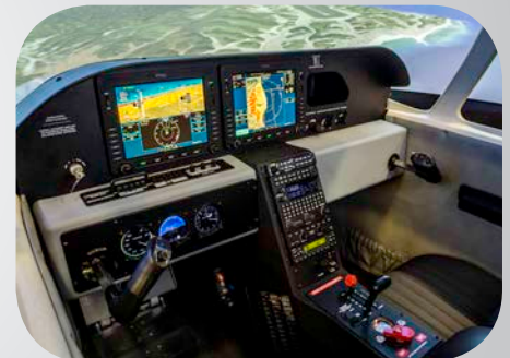
Cirrus SR22 Flight Training Device with fiberglass shell
